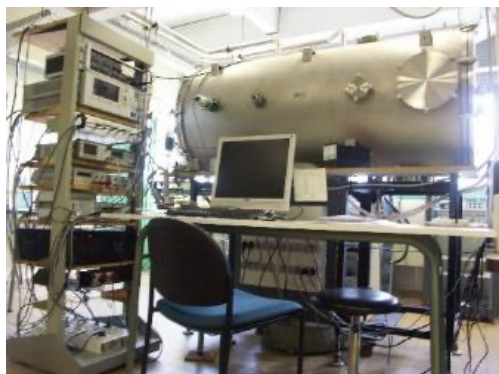
Fourier Transform Microwave Spectrometers 2-20 GHz & sub-millimeterwave spectrometers 50-1500 GHz
